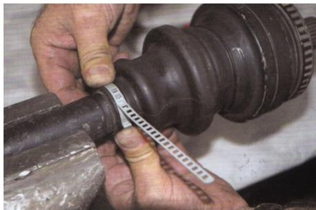
The clamp must be easy to rotate, after inserting in the clamp guide of the axle boot.
